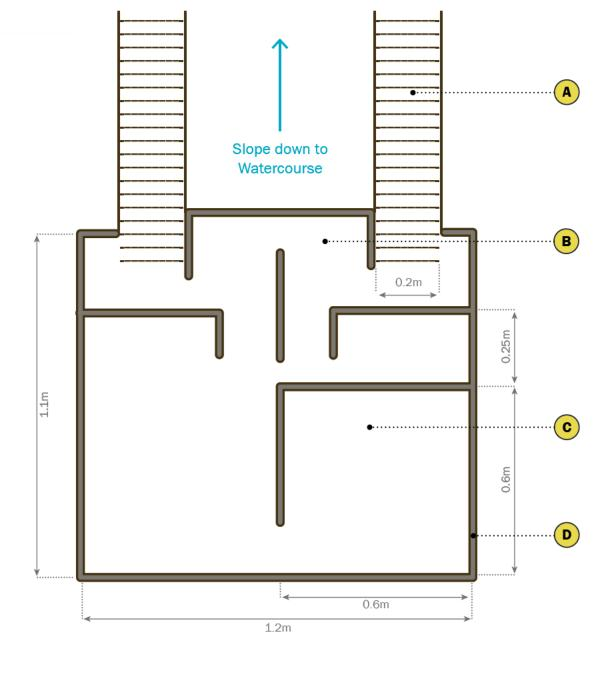
200mm Plastic Culvert Pipe used as access tunnels. One located above the mean water level for use during floods
